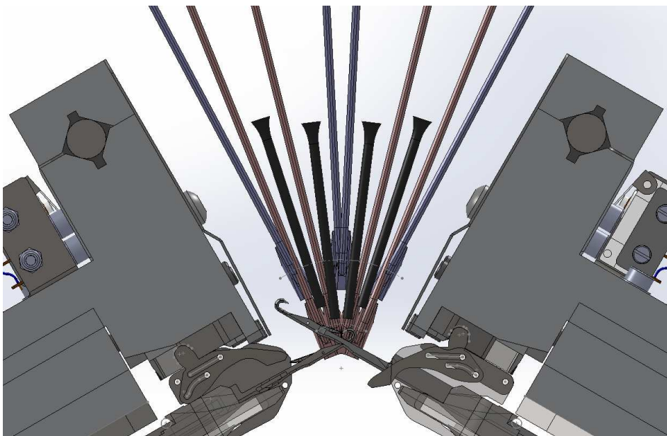
Figure 7: View of the 3D machine knitting area (source: Steiger)
