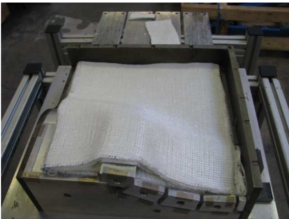
Figure 4: Example of moulding and finished structure (source: Institute of Textile Machinery and High Performance Material Technology, Technische Universität Dresden)
